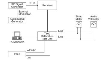
Figure 3.1 T855 Test Equipment Set-up For Short Tuning Procedure
